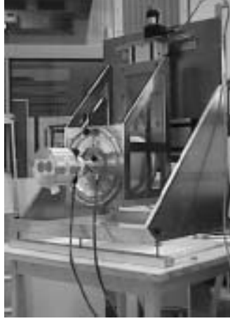
Fig. 2. The SPITS Ge detectors, mounted with their liquid N 2 dewar on the XY-table.
