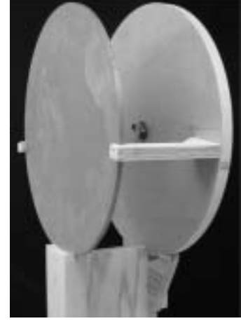
Fig. 3. The Pb disk used as source of extended emission, shown with 88 Y source and mounting device.
