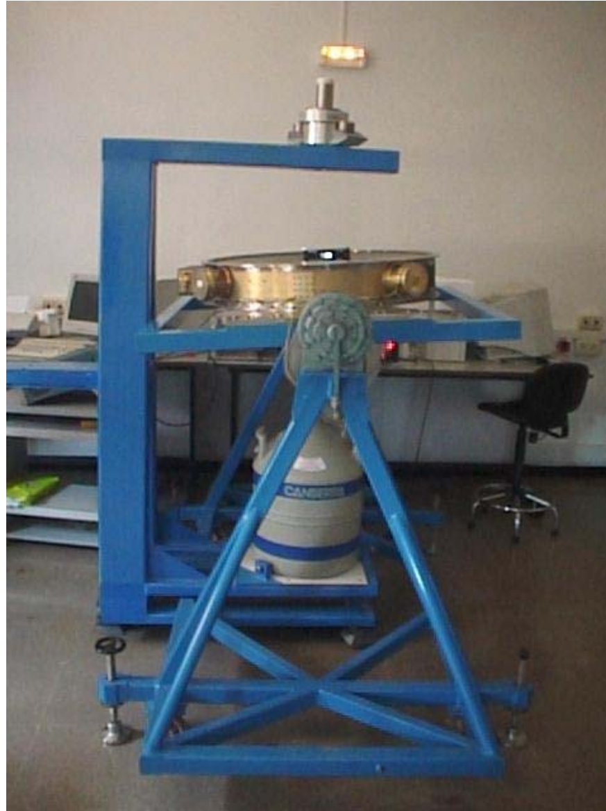
Test equipment used for FINAL STM PSAC transmission measurements
