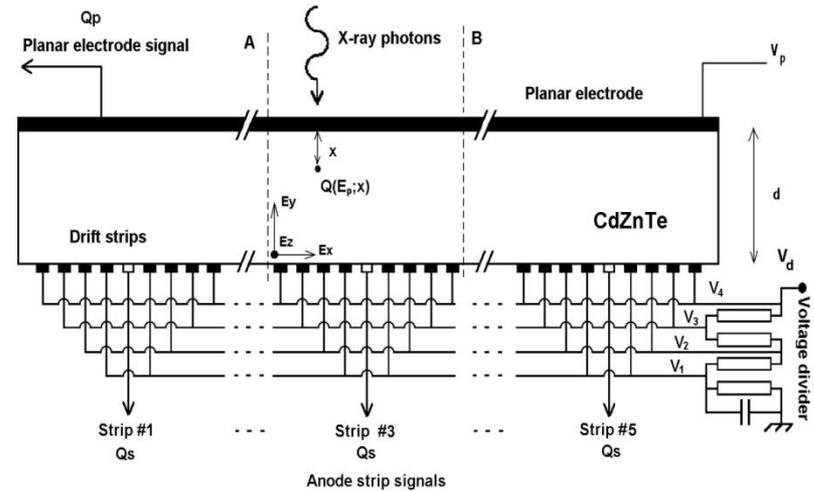
The DTU drift detector with wire connections
