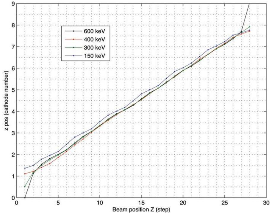
The measured beam position dependence of the actual beam position in the Z direction.
