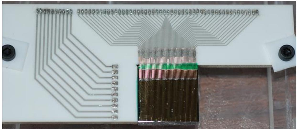
3DCZT prototype (CZT detector: 20 mm x 20 mm x 5 mm).
