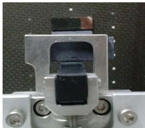
Holder: 3 out of 6 side of the crystal are kept free
